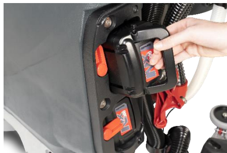
NX300 battery hot-swapping provides the opportunity for continuous cleaning
